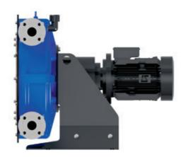
The I43 and I55 models complete the PeriBest peristaltic pump line with a flow rate range between 1,000 and 17,000 I/h. This can be extended by means of a double-head pump up to 34,000 I/h. These two models are perfect for dosing operations of all types of product, where, thanks to the excellent flow rate control, to the constant flow rate in variable pressure applications and to the gentle pumping, accuracies of up to  $\pm 1\%$  can be achieved.
